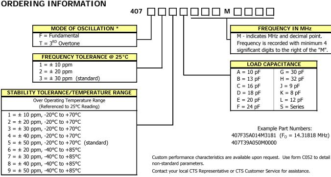
\* Prior to 11/7/06 the part number format did not contain this designator. These "Old Format" numbers (008-0261-0 Rev. E) are still valid with frequencies less than or equal to 48.0000 MHz as Fundamental Mode designs. Frequencies above 48.0000 MHz will be Third Overtone designs. Refer to PCM-1211 for more details.
